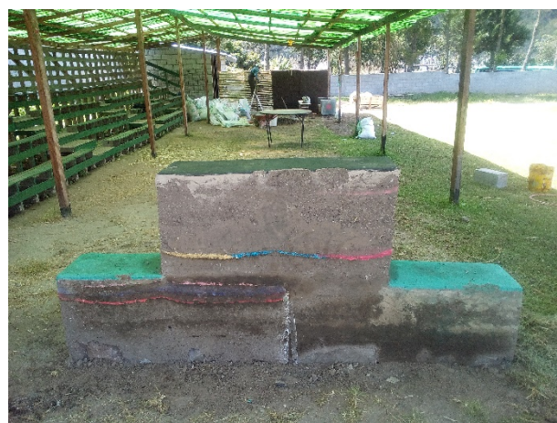
rammed earth example
